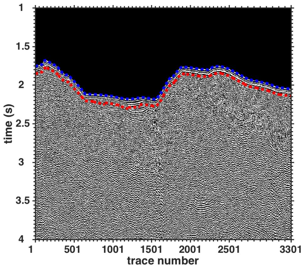
Fig. 1. Section of the seismic profile located in the geographic coordinates (25.10763°N, 109.93275°W) to (25.01640N, 109.74953W) in Farallon Basin. SBR is indicated in dashed blue curve and BSR in dashed red curve.
